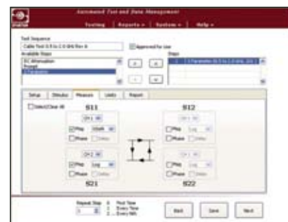
▲ Fig. 1 The Spartan Test Sequence Editor used to define the test procedure.
